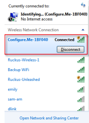
FIGURE 27 Connect to "Configure.Me-[xxxxxx]" WLAN, then launch a web browser
